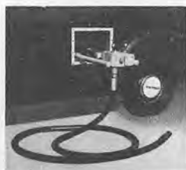
Mounted Operator Equipped with Pipe Tapping Attachment.
