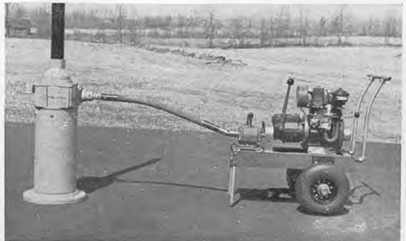
F-5060 Floorstand operated by Portable Gatender
