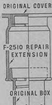
Application of F-2510 Repair Extension
