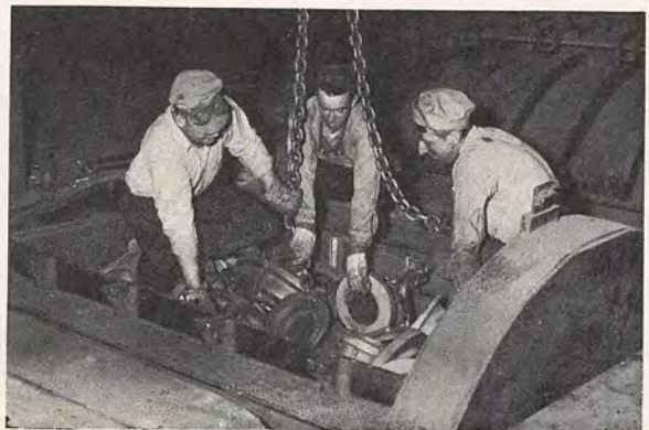
Castings are cleaned in tumbling barrels and all fins are chipped and ground off before shipment.
