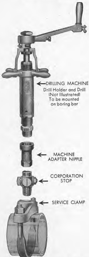
Assembly of Drilling Machine and Sundries To Service Clamp on Main
