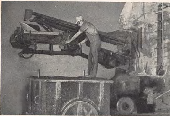
Preparing flask with a mechanical sand slinger.
